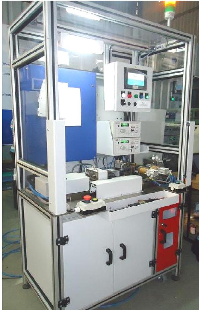
**Application :** EOT – Leak and Performance testing for Brake system pump
