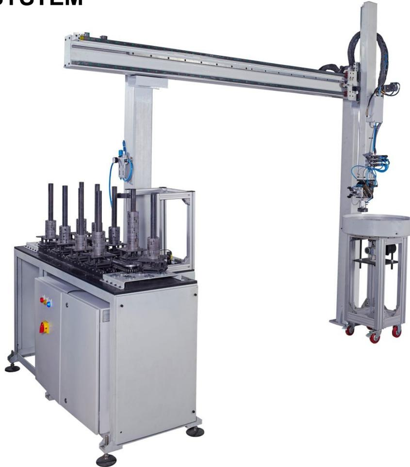
**Application :** Loading and Unloading system of synchro hub from stacker to CNC Machine
