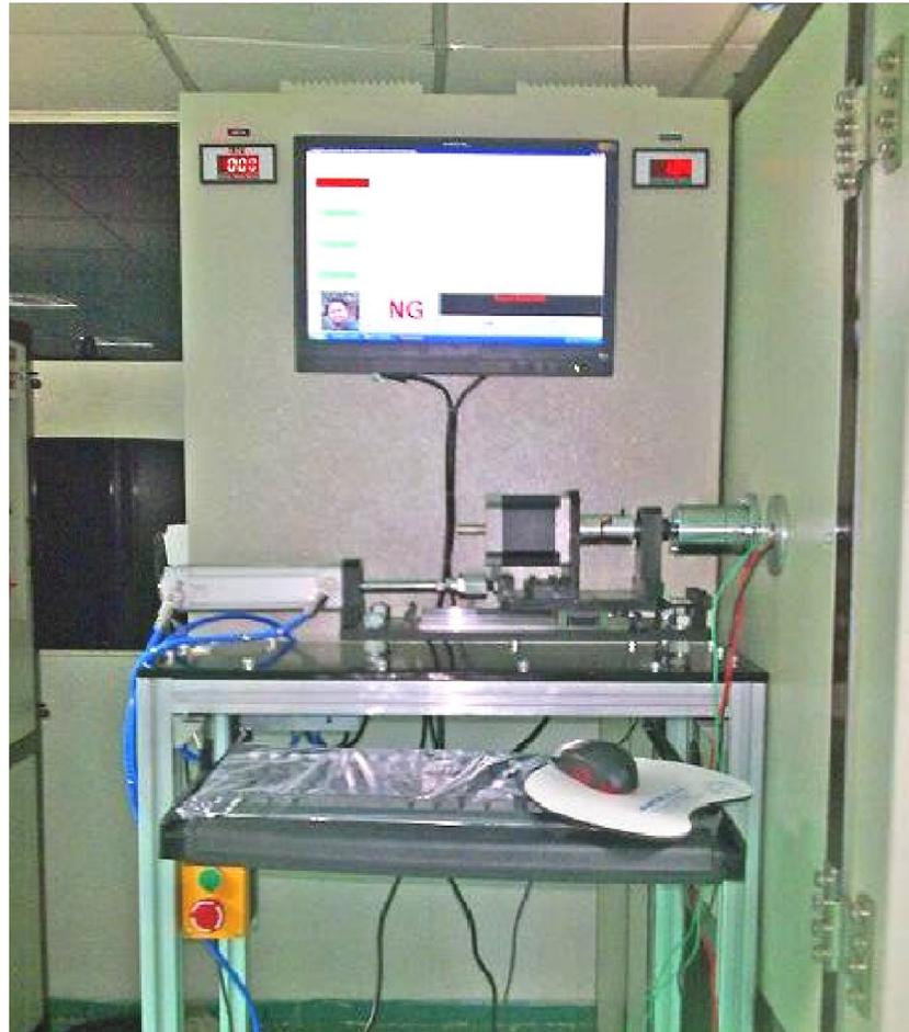
**Application:-**Ignition Switch endurance testing in environmental chamber.
