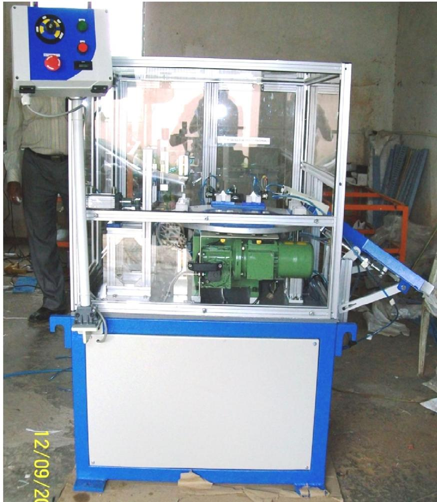
**Application:-** Refrigerator door switches continuity testing & ok-not ok marking.
