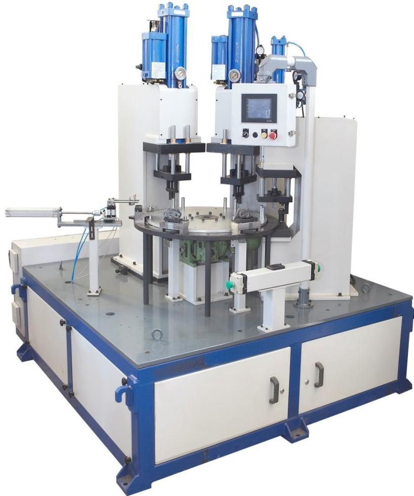
**Application** – Rivet Loading & riveting in to bracket
