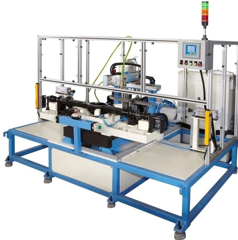
**Application :** Robotic RTV Application and Oil Seal pressing
